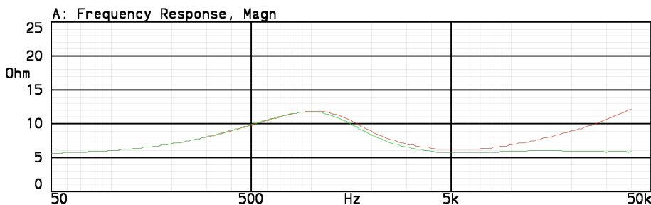
Impedance • with and without impedance correction circuit
